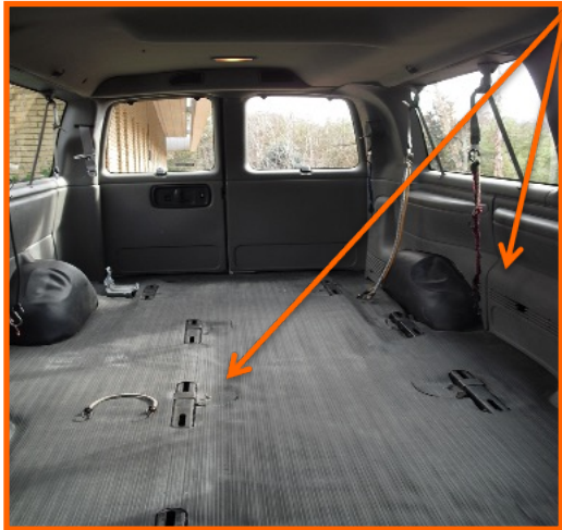
Washable rubber mat and plastic side walls
